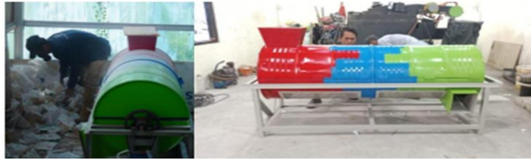
Fig. 3: POJA-PETA Plastic Waste Drying Machine
