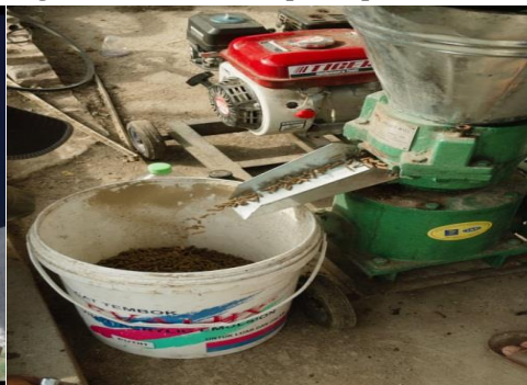
Fig 9. Practical operation of pellet making machine
