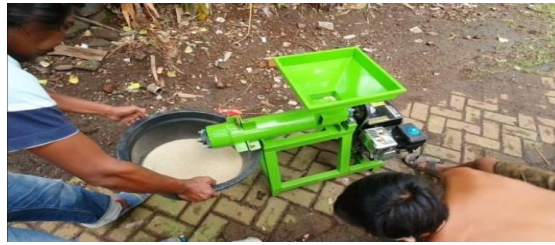
Fig. 3. Grinding dry ingredients using a flouring machine.
