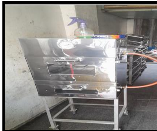
Fig 3. 3 Rack 1 Door Electric Type Oven Machine with Gas Fuel To Dry Herb Ingredients In The Form Of Simplicia, So It's Faster And Evenly
