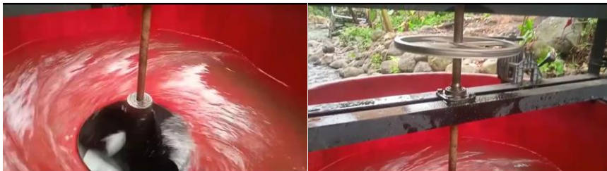
Fig 10. Trial hydro vortex turbine
