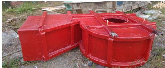
Fig 9. Turbine Tub Maximum Capacity of 1000 Watts
