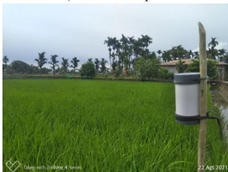
Fig 6. Application of automatic bird repellent in paddy fields
