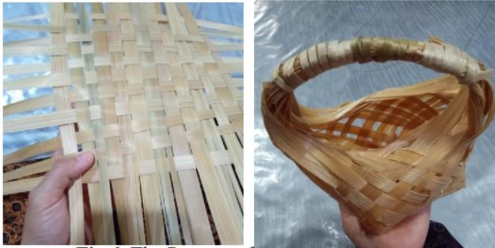
**Fig 6.** The Process of Weaving Bamboo Manually
