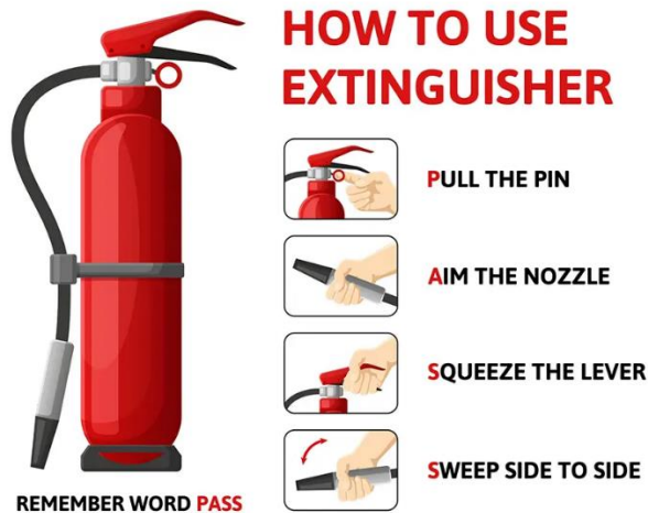
Fig 6. How to Use a Fire Extinguisher
