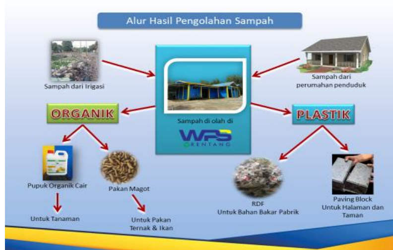
Fig 5. The downstreaming of processed waste products, including RDF, liquid fertilizer, and maggot feed
